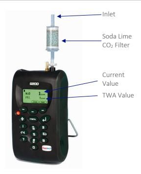
The G200 analyser is specifically designed to safety check background zone levels of  $N_2O$  (0-1,000ppm) in medical applications. This instrument measures the long term exposure to  $N_2O$  gas along with the TWA (time weighted average), leak detection for  $N_2O$  storage. It is a dual purpose background analyser or personal analyser and is highly portable.
