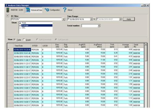
Figure 4 - Example of Data recorded on the Analyser in Person mode, and then ADM calculating the TWA and
