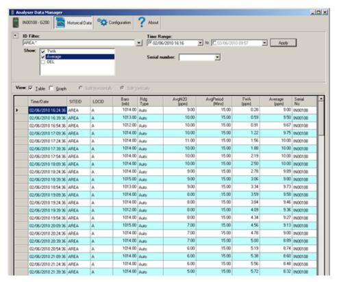
Figure 3 - Example of Data recorded on the Analyser in Area mode, and then ADM calculating the TWA and
