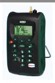
The G210 analyser is specifically designed for highly accurate measurement and verification of the quality of piped  $N_2O$  and  $O_2$  gases in hospitals. This instrument enables up to four gases to be measured, easy user calibration, quick verification of gas quality, user maintained site and sample point IDs for monitoring as well as identification of contaminants CO and  $CO_2$ .
